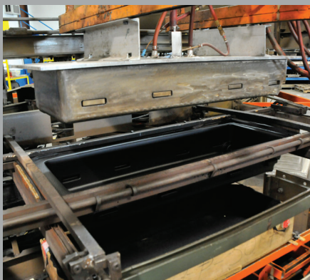
Vacuum mold for keyboard case.
