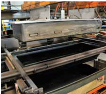
Vacuum mold for keyboard case
